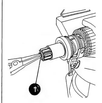
Disassembling overrunning-clutch drive
